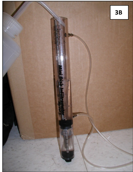
Figure 3. Filling the infiltrometer with water. A. First the tubing is connected to the fittings on the infiltrometer (see section 3.3). Then the upper stopper is removed from the infiltrometer, the chamber is filled, the top replaced, and the tension selection tube pushed as far down as possible so that no water will leak out. B. The infiltrometer is then inverted, the bottom stopper with the porous disk removed, and filled with water. Trapped air prevents water from entering the tubing during this step. After turning the infiltrometer right side up, the tension selection tube can be set to the desired level for beginning the test.
