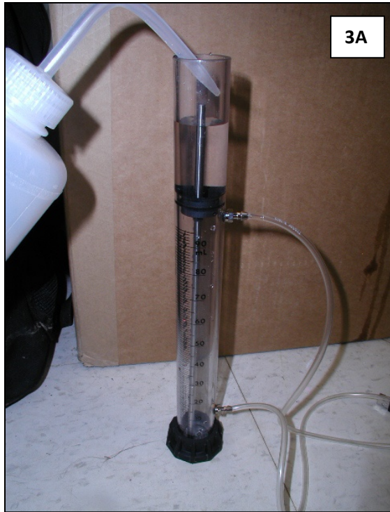
Figure 3. Filling the infiltrometer with water. A. First the tubing is connected to the fittings on the infiltrometer (see section 3.3). Then the upper stopper is removed from the infiltrometer, the chamber is filled, the top replaced, and the tension selection tube pushed as far down as possible so that no water will leak out. B. The infiltrometer is then inverted, the bottom stopper with the porous disk removed, and filled with water. Trapped air prevents water from entering the tubing during this step. After turning the infiltrometer right side up, the tension selection tube can be set to the desired level for beginning the test.
