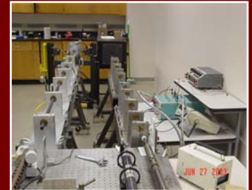
Figure 5. The Split Hopkinson Pressure Bar Set Up @ UMBC
