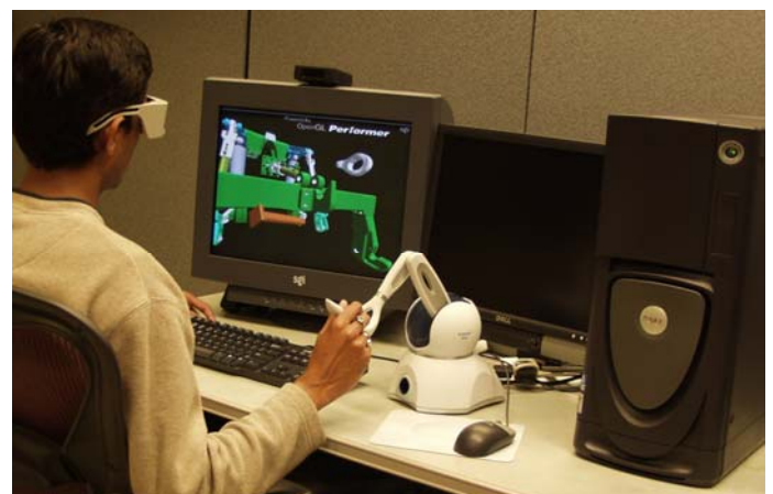
Figure 2: Application Hardware Setup (User performing assembly with PHANToM ® Omni device while viewing parts in stereo using LCD shutter glasses and emitter)
