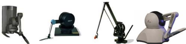
Figure 3: PHANToM ® Desktop, PHANToM ® 1.5, PHANToM ® 3.0 and PHANToM ® Omni, by SensAble Technologies (Images courtesy of Novint Technologies)
