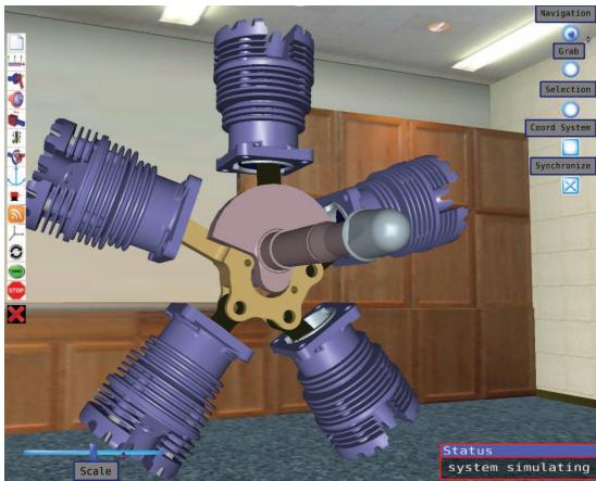
Figure 12. Aircraft engine assembly imported in VRMDS
