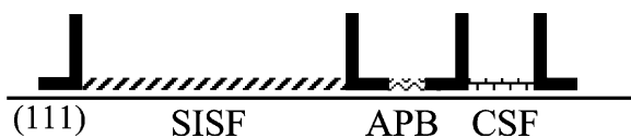
Fig. 1. Planar dissociation of a superdislocation ( \mathbf{b} = < 1 0 1 \rangle ) into four Shockley partial dislocations, a superlattice intrinsic stacking fault (SISF), an antiphase boundary (APB), and a complex stacking fault (CSF).
