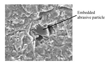
a) A micrograph of the treated surface
