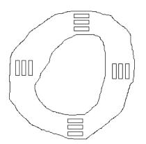
Figure 1: Orientation of specimens obtained from the middiaphysial sections of bovine bone.
