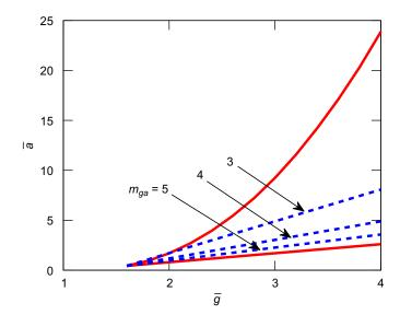
**Fig. 2.** Stability limits of normalized gain  $(\overline{g})$  vs. normalized absorption  $(\overline{a})$  for the SIT modelocked QCL design of Fig. 1. The laser is stable when operates between the two solid (red) curves. The dashed (blue) lines show the operating lines with different  $m_{ga}$ . (For interpretation of the references to color in this figure caption, the reader is referred to the web version of this article.)
