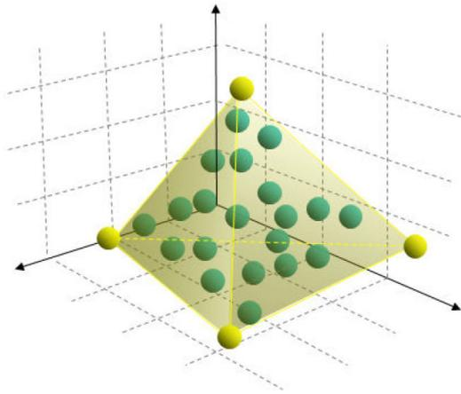
**Figure 7.** The N-FINDR algorithm inflates a simplex with maximum volume using the pixels available in the input hyperspectral data. After a random initialization, it tries all pixels in each endmember position until the combination with maximum volume is found.
