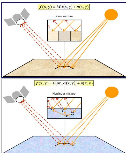
Figure 3. Linear (top) vs nonlinear (bottom) unmixing.
