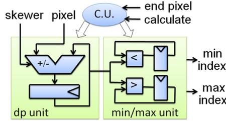
Figure 4. Hardware architecture of a dot product processor.
