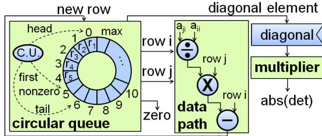
Figure 7. Hardware architecture of the  $\text{abs}(\det)$  module.
