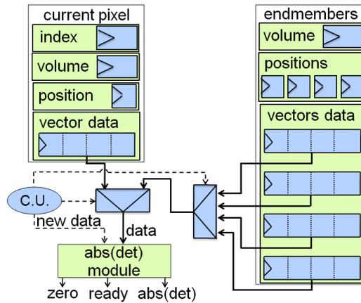
Figure 6. Hardware architecture to implement the N-FINDR algorithm.
