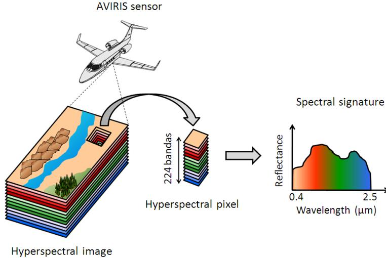
Figure 1. The concept of hyperspectral imaging.
