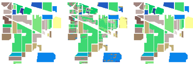
Fig. 5. Classification maps obtained for the AVIRIS Indian Pines scene with 10% randomly selected training samples per class. (Left) Original ground truth. (Center) Classical 2DCNN model. (Right) Proposed MCMs+2DCNN model.
