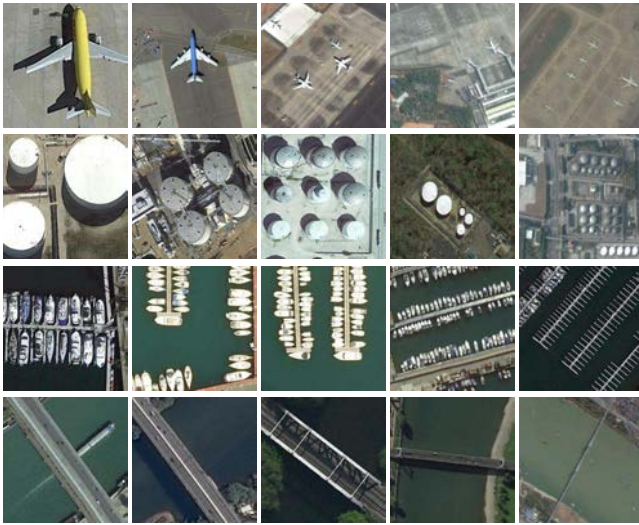
Fig. 1. Example to illustrate the problem of LSV in RSSC. From top to bottom, we can observe the existing scale variability between objects belonging to the same class in the following classes: airplane (top row), storage tank (second row), harbor (third row), and bridge (bottom row), respectively.
