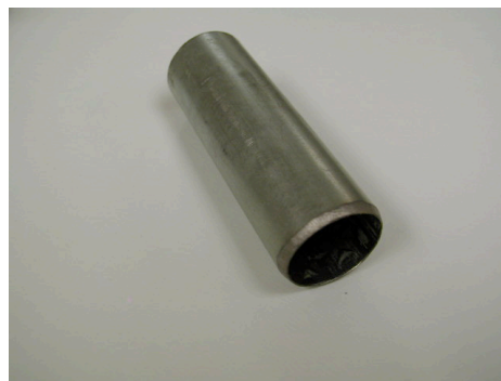
Figure 2. Bulk density core sampler made from 1/2" electrical conduit.
