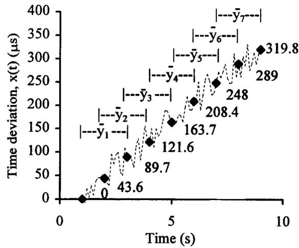
**Figure C.2—Computation of  $\bar{y}_k$ s for overlapped estimates**
