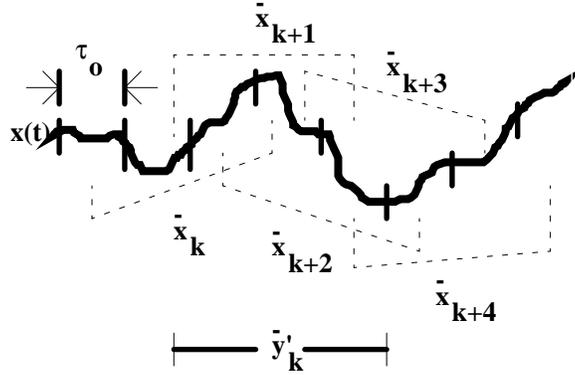
Figure C.3—Method for calculating  $\bar{x}_k$ s, and  $\bar{y}'_k$ s for Mod  $\sigma_y(\tau)$
