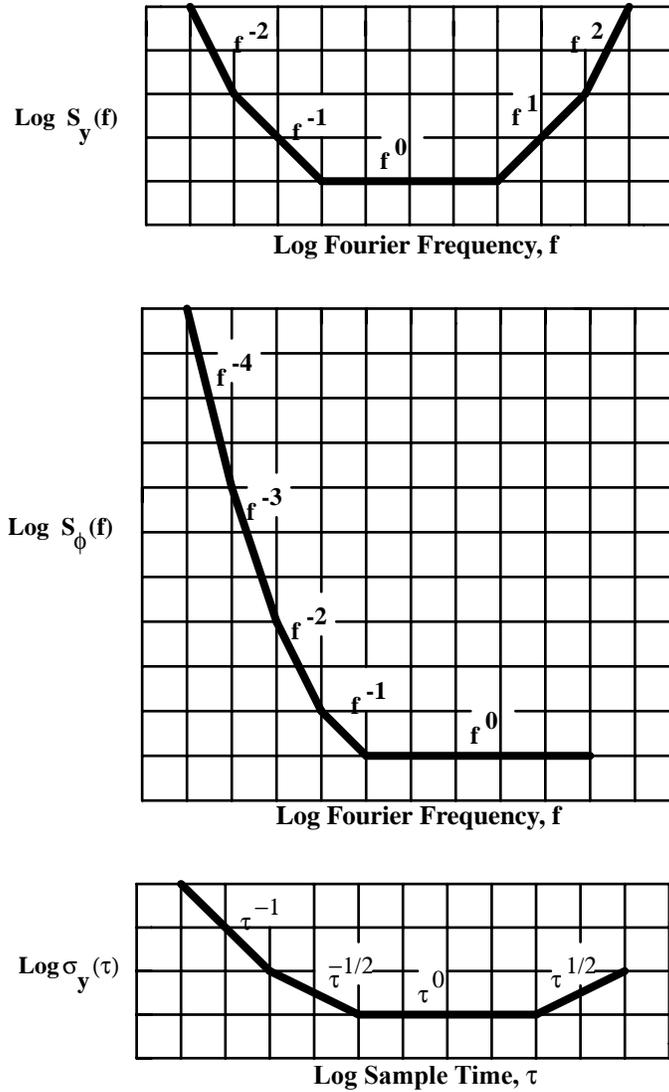
Figure B.1—Slope characteristics of the five independent noise processes
