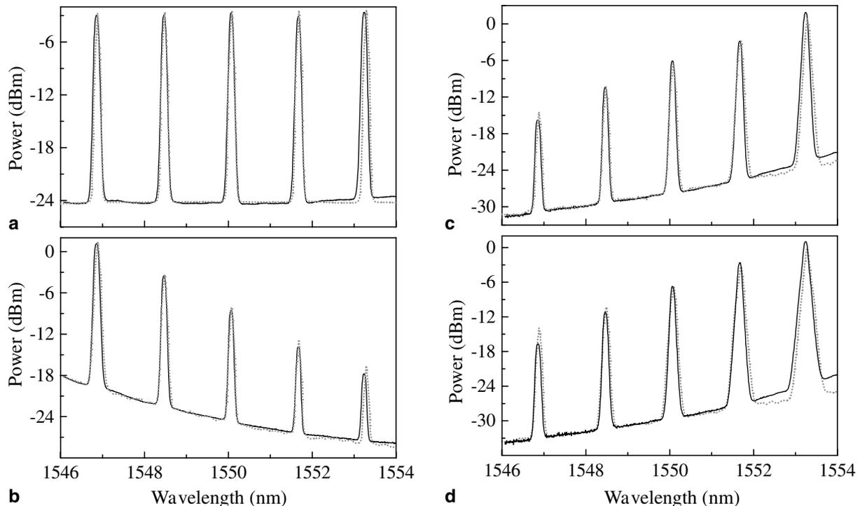
Fig. 6. Spectra for four different settings of the Raman pump power and  $\Delta_{\text{EDFA}}$  after 1700 km of propagation. Experimental results are shown as solid curves while theoretical results are shown as dotted curves. In (a) the pump values are set so that the system has 0 dB net gain and no tilt. In (b), there is excess EDFA gain. In (c), excess Raman gain is used to compensate the lower EDFA gain. In (d), we show channel broadening when increasing the amount of Raman and EDFA gain.
