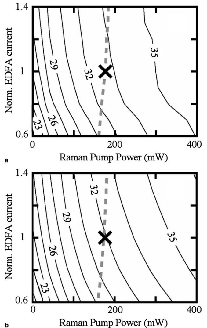
Fig. 5. Contour plots of the OSNR of the center channel in dB: (a) experimental values and (b) simulated values, as a function of the Raman pump power and  $\Delta_{EDFA}$ . The X denotes the pump values for which the system is transparent (net gain is 0 dB) and has no tilt. The dashed curve represents the parameter set corresponding to no tilt (see Fig. 3).
