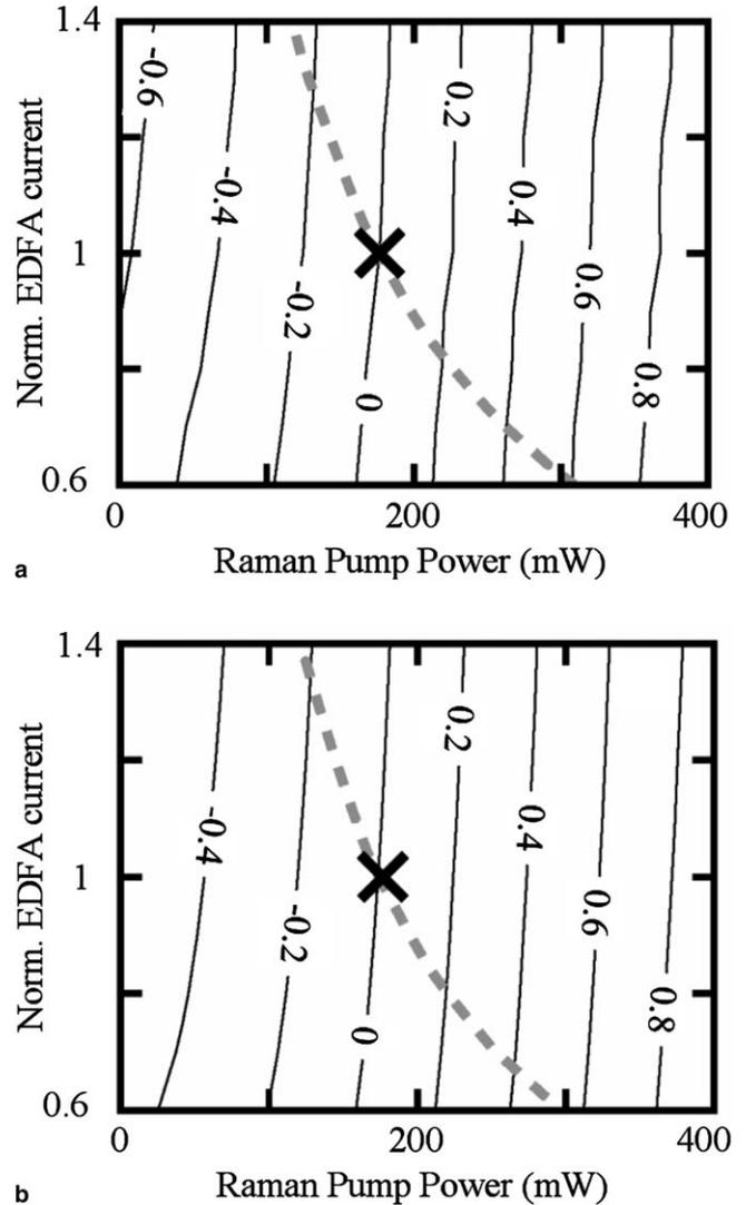
Fig. 3. Contour plots of the signal tilt in dB/nm: (a) experimental values and (b) simulated values, as a function of the Raman pump power and  $A_{\text{EDFA}}$ . The X denotes the pump values for which the system is transparent (net gain is 0 dB) and has no tilt. The dashed curve represents an average of  $-3$  dBm per channel.
