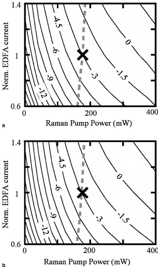
Fig. 4. Contour plots of the mean output power in dBm: (a) experimental values and (b) simulated values, as a function of the Raman pump power and  $\Delta_{EDFA}$ . The X denotes the pump values for which the system is transparent (net gain is 0 dB) and has no tilt. The dashed curve represents the parameter set corresponding to no tilt (see Fig. 3).
