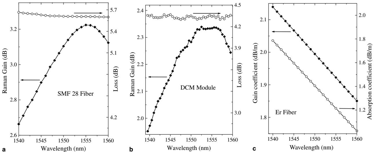
Fig. 2. Gain and loss characteristics of the fiber in the loop: (a) gain and loss for the SMF-28, (b) gain and loss for the DCM and (c) gain and absorption coefficients of the erbium fiber used in the EDFAs in the loop.
