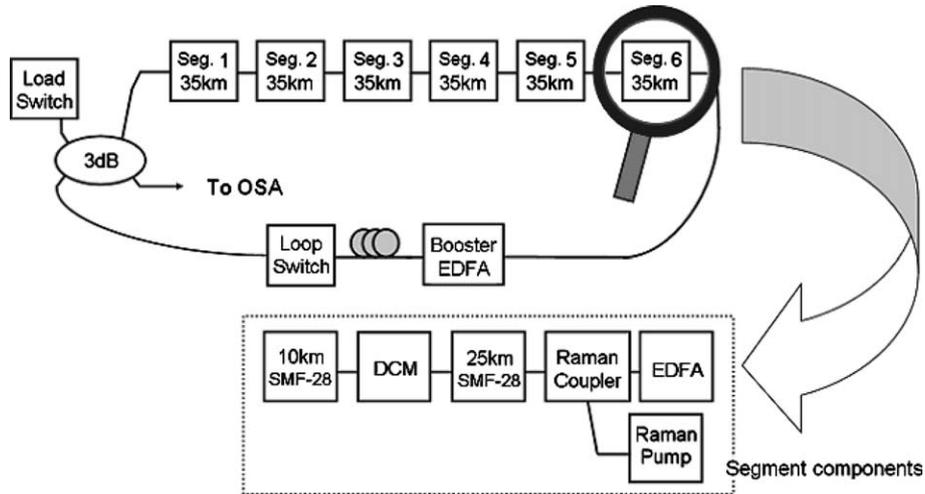
Fig. 1. Schematic of our 210 km recirculating fiber-optic loop.
