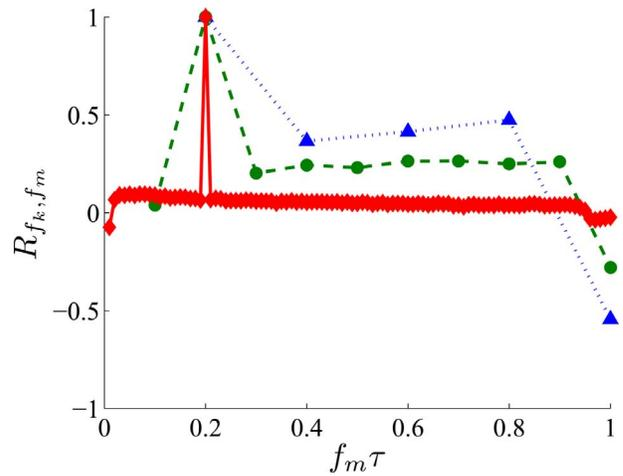
Fig. 4. (Color online) Cross correlation between the normalized Fourier coefficients  $\xi_{\text{rf}}(f_k=1/5\tau)$  and  $\xi_{\text{rf}}(f_m)$  calculated for three different measurement durations:  $T=1/f_k$  (dotted triangles),  $T=2/f_k$  (dashed circles), and  $T=20/f_k$  (solid diamonds).
