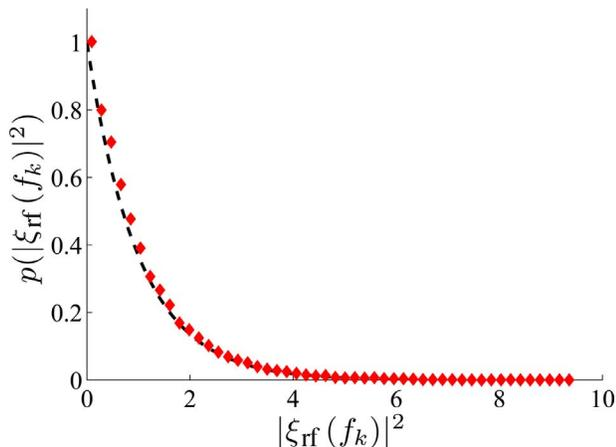
Fig. 3. (Color online) Distribution of the normalized rf spectrum,  $|\xi_{\text{rf}}(f_k)|^2$ , at a frequency  $f_k\tau=1/10$  calculated from 30,000 runs. An exponential distribution with an average of 1 is added for comparison (dashed curve).
