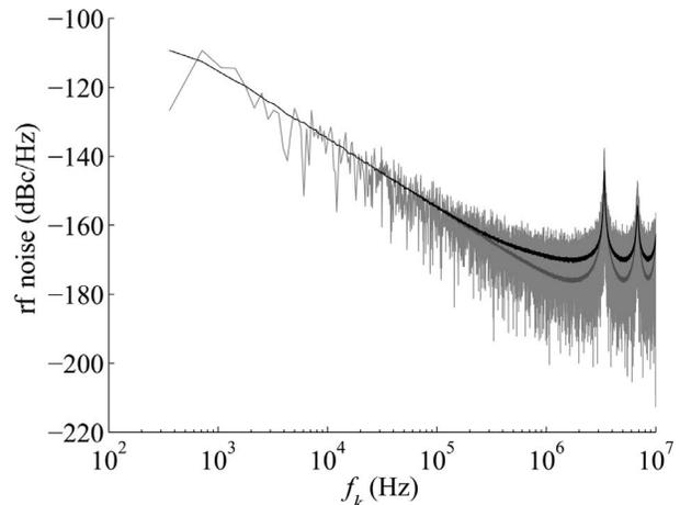
Fig. 1. Radio frequency spectrum  $S_{\text{rf}}(f_k)$  as a function of the frequency offset from the carrier frequency. The spectrum was calculated from a single simulation run with a measurement duration of  $T = 2.8$  ms (light gray curve). The rf spectral density (black curve) and the phase spectral density (dark gray curve) were calculated by averaging the results over 350 runs.
