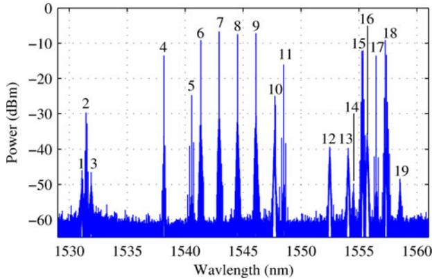
Fig. 8. 10 MHz resolution optical spectrum of test WDM signal plan. This plan includes OOK, BPSK and QPSK signals with data rates ranging from 4.25 to 42.67 Gb/s, dispersion ranging from  $-2600$  to  $+800$  ps/nm and OSNRs of 13 to  $>30$  dB-0.1 nm.
