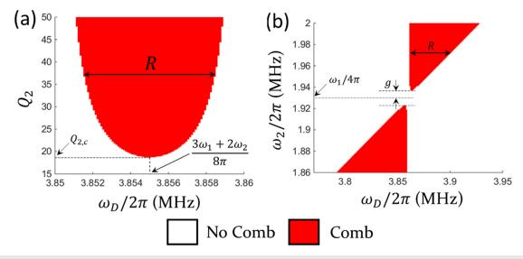
**FIG. 4.** Regions for generation of phononic frequency combs. (a) Quality factor of mode 2 vs drive frequency. (b) Resonance frequency of mode 2 vs drive frequency. System parameters: (a)  $\frac{\omega_1}{2\pi} = 3.86$  MHz,  $Q_1 = 4000$ , and  $\frac{\omega_2}{2\pi} = 1.92$  MHz and (b)  $\frac{\omega_1}{2\pi} = 3.86$  MHz,  $Q_1 = 4000$ ,  $Q_2 = 50$ .
