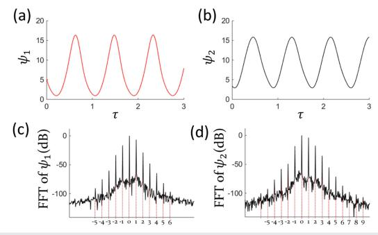
**FIG. 3.** Numerical simulation results for the mode amplitudes, Eqs. (5) and (6), within the phononic frequency comb boundary. Simulation parameters:  $\Delta_1 = 5$ ;  $\kappa = -9$ ;  $\Delta_2 = \frac{\Delta_1}{2} + \kappa$ ;  $\gamma_{21} = 1$ ; f = 20. (a) and (b) Time domain responses. (c) and (d) Corresponding fast Fourier transforms (FFT) showing the existence of phononic frequency combs.
