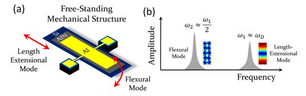
FIG. 1. Micromechanical resonator and phononic frequency comb concept. (a) Micromechanical resonator design used in Ref. 7 to generate phononic frequency combs. A length-extensional mode couples to a flexural mode through a nonlinear strain relationship. (b) Visual description of the mode coupling concept that results in phononic frequency combs, showing two modes where the resonance frequency of one mode is near double that of the other mode.
