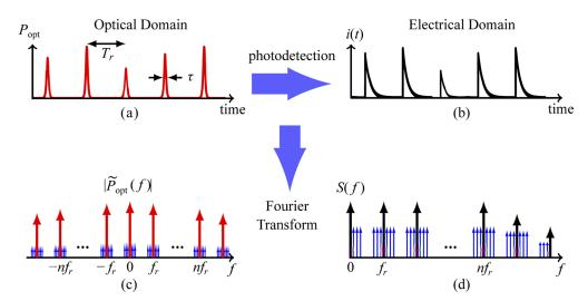
**Fig. 5.** Time and frequency domain depictions of modulated input optical and output electrical pulse trains, where  $T_r$  is the repetition time and  $\tau$  is the pulse duration of the optical signal. (a) Modulated input optical pulse train. (b) Modulated output electrical pulse train. (c) Spectrum of the modulated optical intensity. (d) Power spectrum of the modulated photocurrent. This figure is similar to Fig. 2 in Jamali *et al.*[4].
