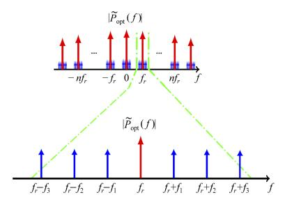
**Fig. 6.** Expanded view of the spectrum of the modulated optical intensity profile. Red arrows show comb lines at harmonics of the repetition frequency. Blue arrows show the comb lines at modulation frequencies  $(nf_r \pm f_1, nf_r \pm f_2, \text{ and } nf_r \pm f_3)$  for each comb line where n is the comb line number. In the expanded view, we show comb lines for n = 1.
