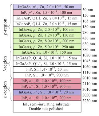
**Fig. 1.** MUTC PD structure [13]. Green indicates the absorption regions, which include an intrinsic region and a *p*-doped region. Red indicates highly-doped InP layers, purple indicates highly-doped InGaAs layers, and white indicates other layers. This figure is the same as Fig. 1 in Hu *et al.*[12].
