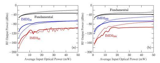
**Fig. 11.** Power at the fundamental frequency  $(nf_r)$ , the IMD2<sub>n</sub> power at the modulated frequency  $nf_r + (f_1 - f_2)$ , and the IMD3<sub>n</sub> power at the modulated frequency  $nf_r + (f_1 - f_2 + f_3)$ . Solid lines show results with bleaching; dotted lines show results without bleaching: (a) n = 20 ( $nf_r = 1$  GHz), (b) n = 200 ( $nf_r = 10$  GHz).
