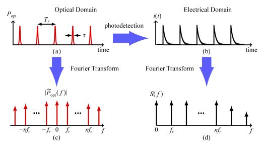
**Fig. 4.** Time and frequency domain depictions of the input optical and output electrical pulse trains, where  $T_r$  is the repetition time and  $\tau$  is the pulse duration of the optical signal. (a) Input optical pulse train intensity profile. (b) Output electrical pulse train. (c) Spectrum of the optical intensity profile. (d) Power spectrum of the photocurrent. This figure is similar to Fig. 1 in Quinlan *et al.*[20].
