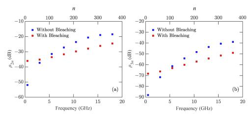
**Fig. 12.** Distortion to signal ratios as a function of comb line frequency and number with and without bleaching for: (a)  $\rho_{2n}$ , (b)  $\rho_{3n}$ .
