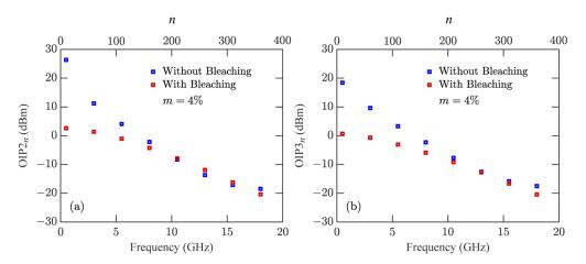
**Fig. 9.** OIP2 $_n$  and OIP3 $_n$  as a function of comb line frequency and number with an average input optical power of 25 mW. (a) OIP2 $_n$ ; (b) OIP3 $_n$ .
