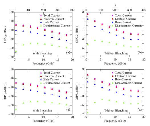
**Fig. 10.** Contribution of different current components to  $OIP2_n$  and  $OIP3_n$  as a function of comb line frequency and number. The magenta, red, blue, and green curves show the contributions of the total, electron, hole, and displacement currents, respectively. (a)  $OIP2_n$  with bleaching, (b)  $OIP2_n$  without bleaching, (c)  $OIP3_n$  with bleaching, (d)  $OIP3_n$  without bleaching.
