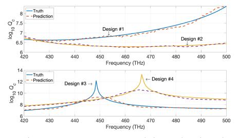
**Figure 6.** True (CMT-determined) vs predicted  $Q_c$  values for two devices without (top) and with (bottom) a peak (referred in the main text as a coupling antiresonance) in the frequency range of interest. In contrast to Figure 3, here we perform an extrapolation study where training is done using CMT-based  $Q_c$  calculations for certain values of *RW* and *W*, and testing is done for *RW* and *W* values outside of the testing range.
